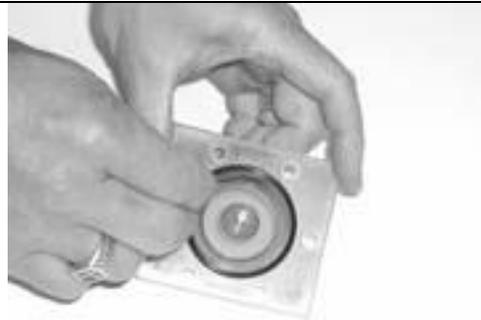
8. Place the rotor in the flow cavity.
