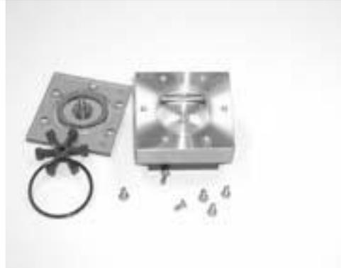
5. Using a soft cloth dampened with water, alcohol or a light detergent solution, clean debris and dirt from the rotor, the stainless steel shaft, the inside surfaces of faceplate and the surfaces of the flow cavity
