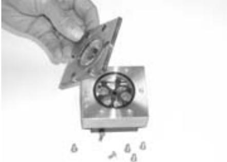
A photograph showing a hand holding the removed faceplate above the flow switch body. The faceplate is a circular metal plate with a central hole. The flow switch body is the square metal block with the circular opening. Six screws are scattered on the surface below the body.                     |
