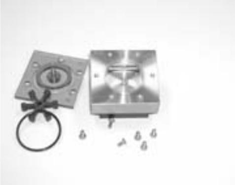
A photograph showing the disassembled components of the flow switch. The faceplate is on the left, the rotor and stainless steel shaft are in the center, and the flow switch body is on the right. The o-ring is also visible on the faceplate. Six screws are scattered on the surface below the body. |
